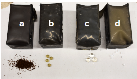
FIGURE 3. Granule Test Samples - a: Coffee granules, b: Rubber beads, c: Hydrated Polyacrylamide Balls, d: Polystyrene balls
