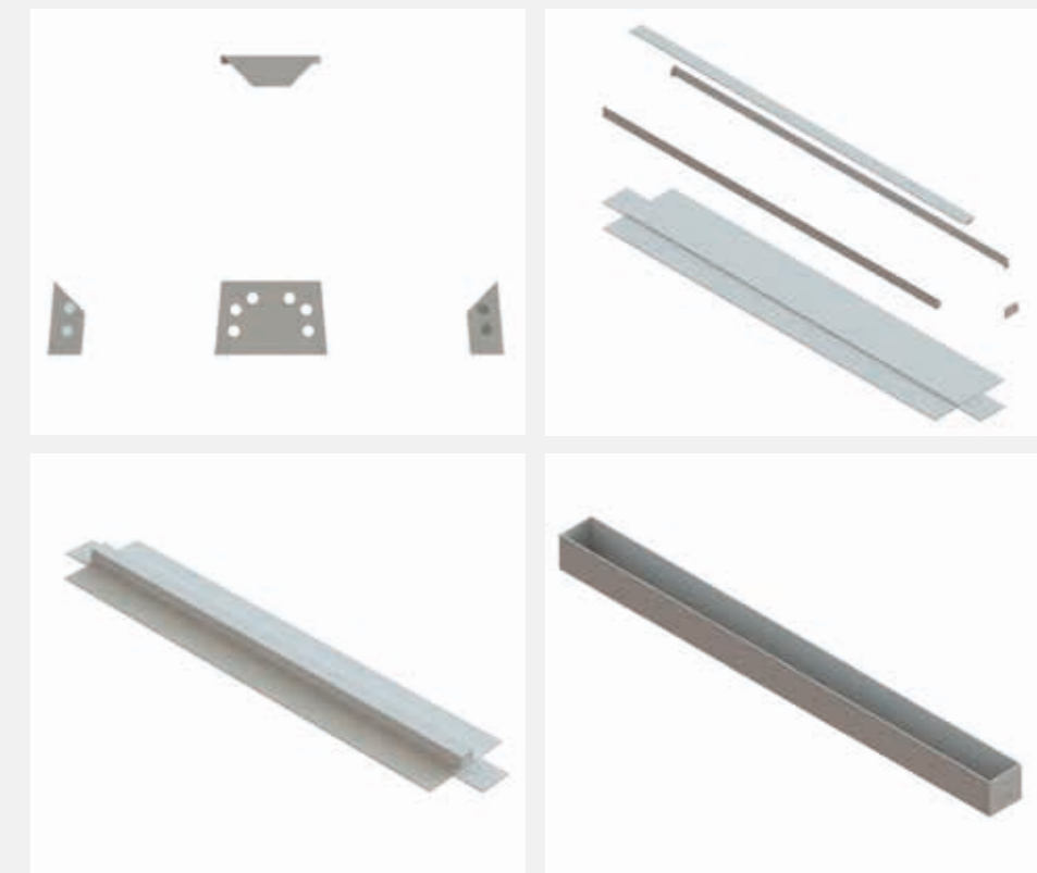
Figure 21 - Low cost collapsible mould design. From top left clockwise - a) Exploded internal mould b) Exploded entire mould c) Entire mould open d) Entire mould closed
