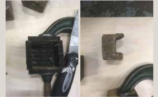
Figure 16 - Laser cut mould and output
