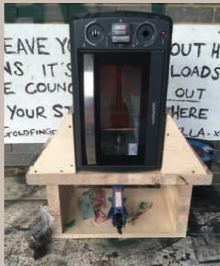
Figure 12 - DIY hot press
