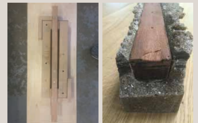
Figure 19 - Plywood mould and output product prior to cleaning.
