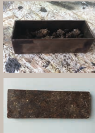
Figure 13 - Metal mould and output tile
