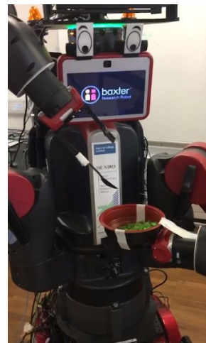
Figure 19 - Scooping from the robot's left end effector
